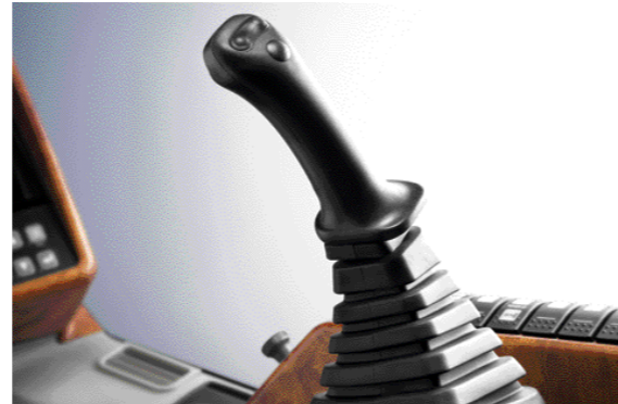
Joystick Grip Additional switches are standard on each joystick for controlling any attachment.
