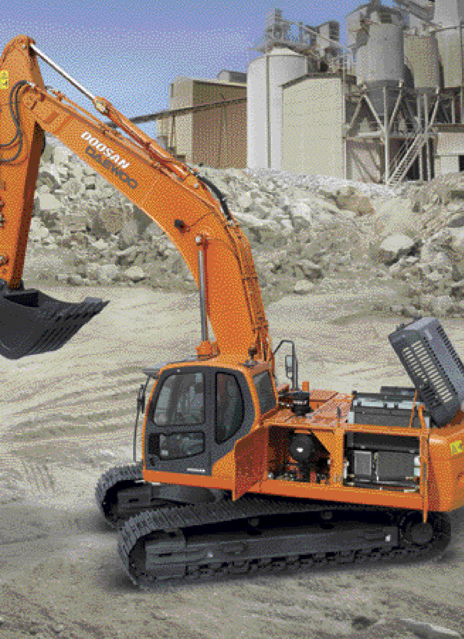
Easy Maintenance Excellent access is provided through the top engine cover and both side panels.
