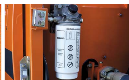
Fuel Filter High efficiency filtration is ensured through a pick-up filter within the tank followed by a primary filter and water separator and one final filtration before entering the common rail delivery system, all driven by a priming and high pressure pump that makes engine starting easy.
